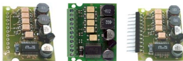
BW1421 / BW1490 with screw terminals with wiring pins
