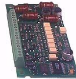
AS-i 4I Module for building automation
