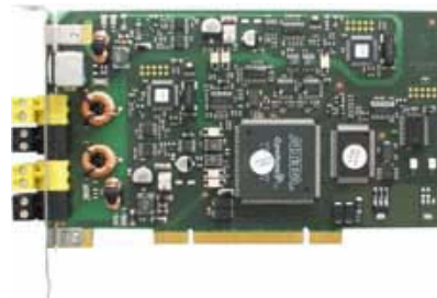
PCI Board with 2 AS-i Masters
